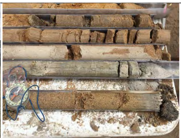
Photograph 17. Core produced from geoprobe rig.
