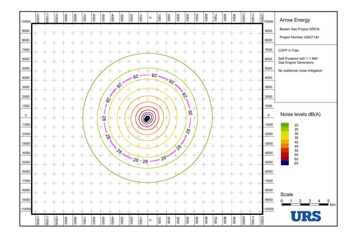
Figure-C-14 Indicative noise level contours: CGPF (5-train) – 1.1 MW local power generators (without additional noise mitigation)
