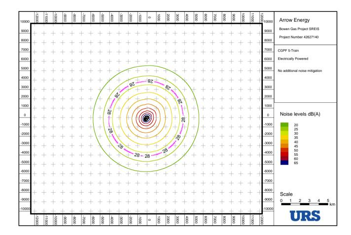
Figure-C-13 Indicative noise level contours: CGPF (5-train) – electrically powered (without additional noise mitigation)
