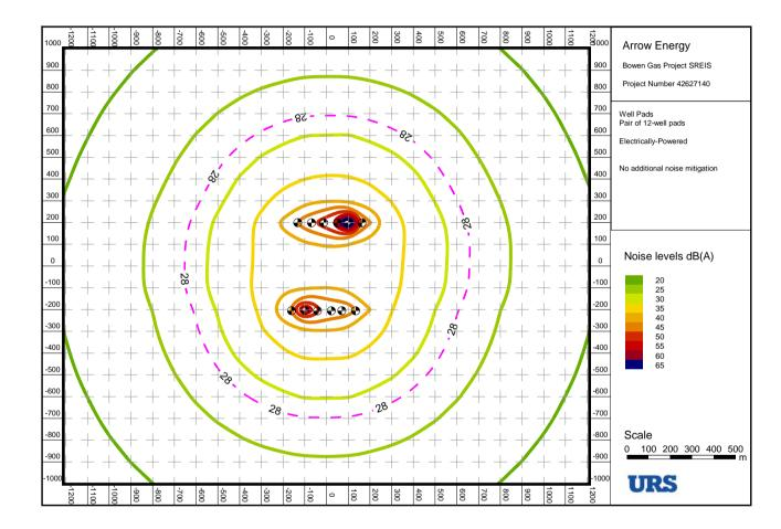
Figure-C-5 Indicative noise level contours: Pair of 12-well pads - electrically powered (without noise mitigation)
