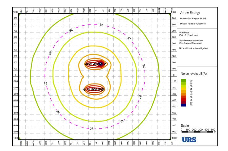
Figure-C-6 Indicative noise level contours: Pair of 12-well pads - local power generation (without noise mitigation)
