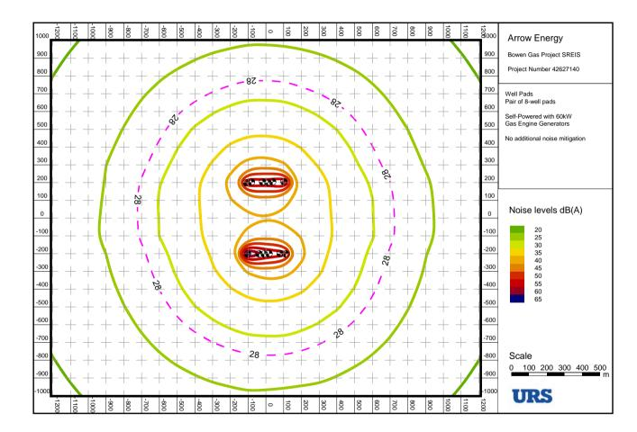
Figure-C-4 Indicative noise level contours: Pair of 8-well pads - local power generators (without noise mitigation)
