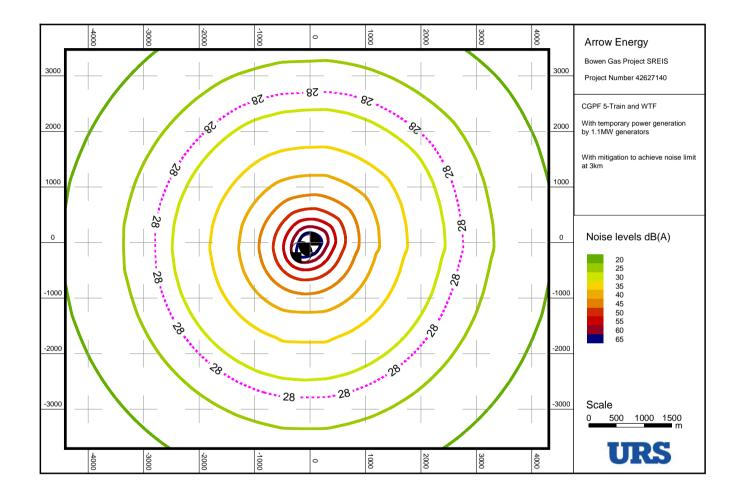
Figure-E-5 CGPF 5-train and WTF - temporary power by 1.1 MW generators - with mitigation to achieve limit at 3 km
