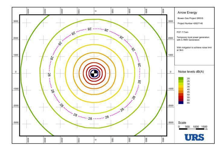
Figure-E-3 FCF 7-train with temporary local power generation by 5.7 MW gas turbines, with mitigation to achieve noise limit at 3 km
