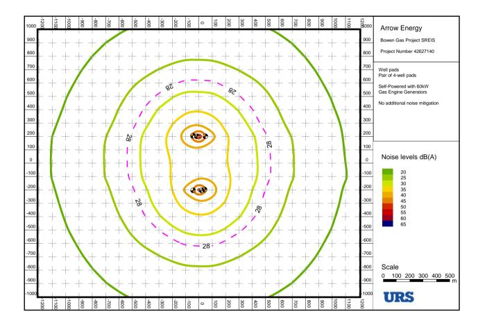
Figure-C-2 Indicative noise level contours: Pair of 4-well pads - local power generators (without noise mitigation)
