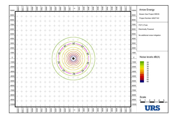
Figure-C-7 Indicative noise level contours: FCF (3-train) – electrically powered (without additional noise mitigation)
