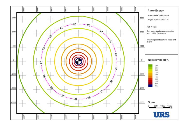
Figure-E-2 FCF 7-train with temporary local power generation by 1.1 MW gas engines, with mitigation to achieve noise limit at 3 km
