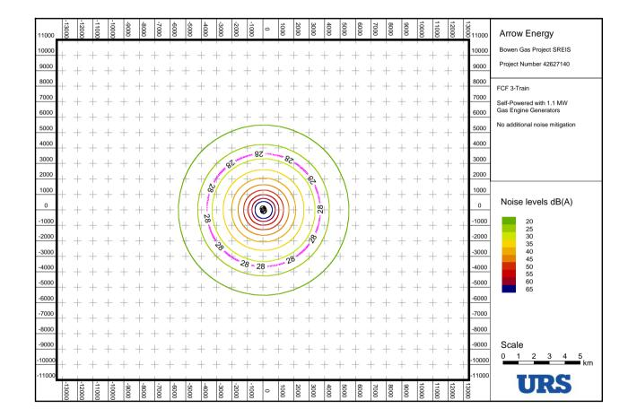
Figure-C-8 Indicative noise level contours: FCF (3-train) – 1.1 MW local power generators (without additional noise mitigation)
