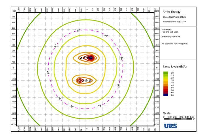
Figure-C-3 Indicative noise level contours: Pair of 8-well pads - electrically powered (without noise mitigation)
