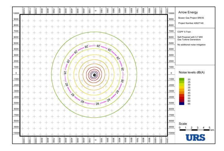
Figure-C-15 Indicative noise level contours: CGPF (5-train) – 5.7 MW local power generators (without additional noise mitigation)
