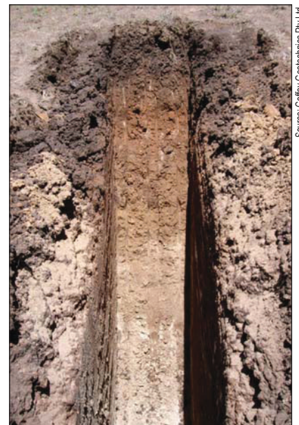
Plate 12.3 CTP1 test pit excavation exposing brown Dermosol soil profile
