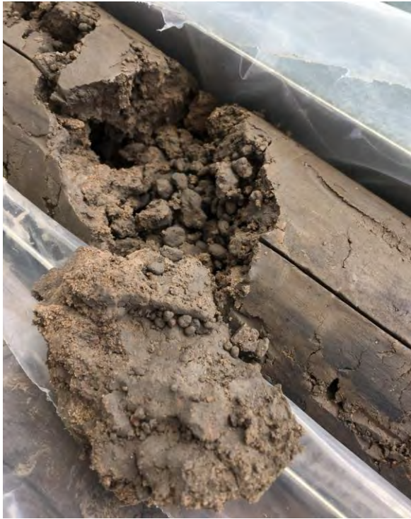
Figure 36. Clay pebbles in open fissures at 2m; and underlying clayey sand comprising a very moist vadose zone inferred to be the horizon of predominant soil moisture uptake by trees.
