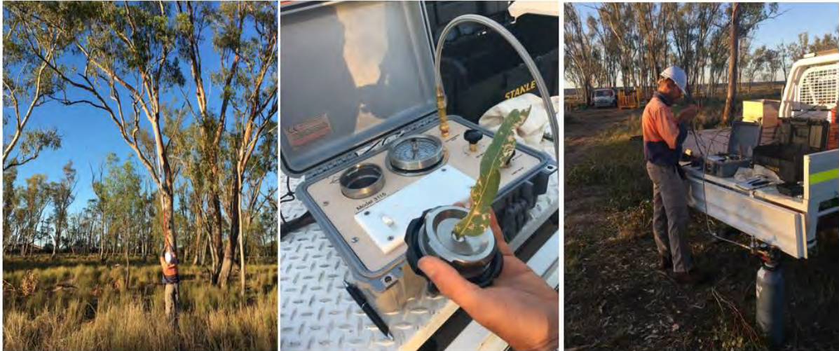
Figure 19. Leaf collection, insertion of the leaf petiole into the grommet for sealing in the pressure chamber and measurement of water potential.
