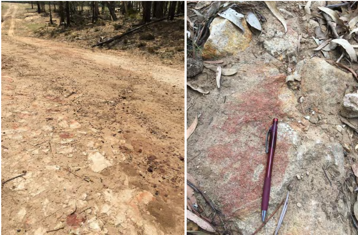
Figure 54. Weathered sandstone outcrop within the nearby road (drilling site visible in background across the dry creek bed) and adjacent to the road in a low cutting.
