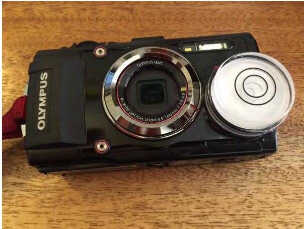
Figure 20. Camera mounted with a bullseye level for canopy photography.
