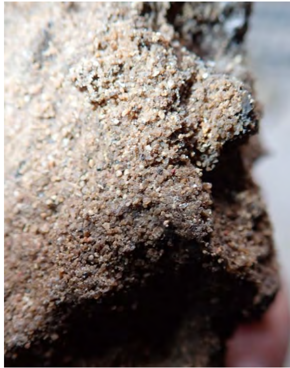
Figure 36. Clay pebbles in open fissures at 2m; and underlying clayey sand comprising a very moist vadose zone inferred to be the horizon of predominant soil moisture uptake by trees.
