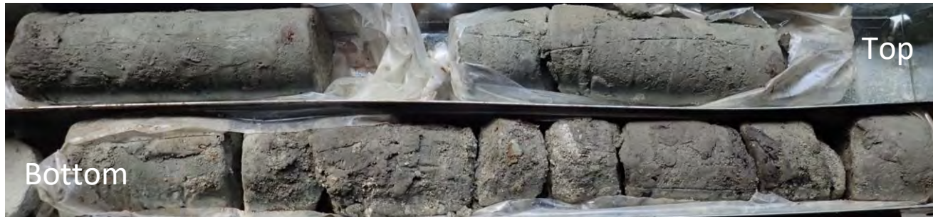
GB20A 24 – 27m (1.5m core loss – likely coal)
