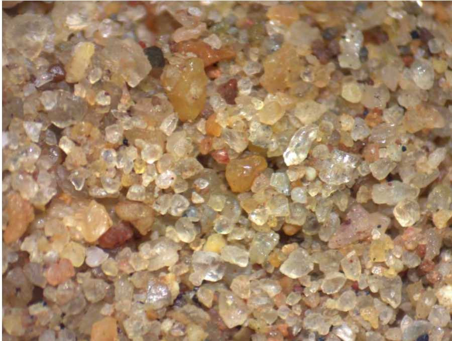
Figure 38. Poorly sorted sand unit encountered in Long Swamp 35 (Photo of sample collected at 30m depth).
