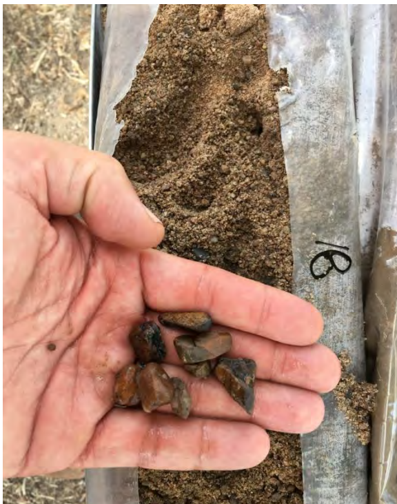
Figure 37. Dry gravelly sand alluvium at 18m along the angle core (15mGL)
