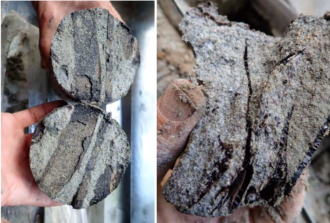
Figure 55 . Coal fragments in sandstone core from Glenburnie 20 at 22.5-24m.
