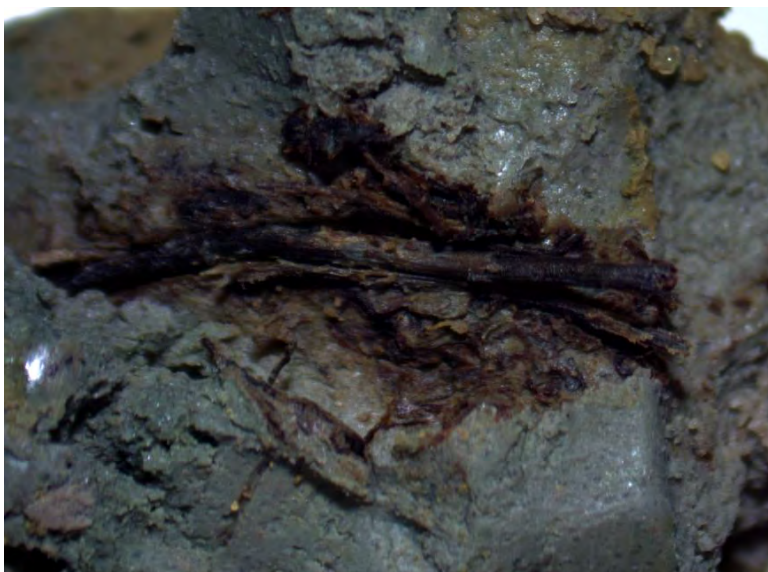
Figure 27. Fibrous tree roots to 3mm thickness in fissured sandy clay at 4m depth in LB31a
