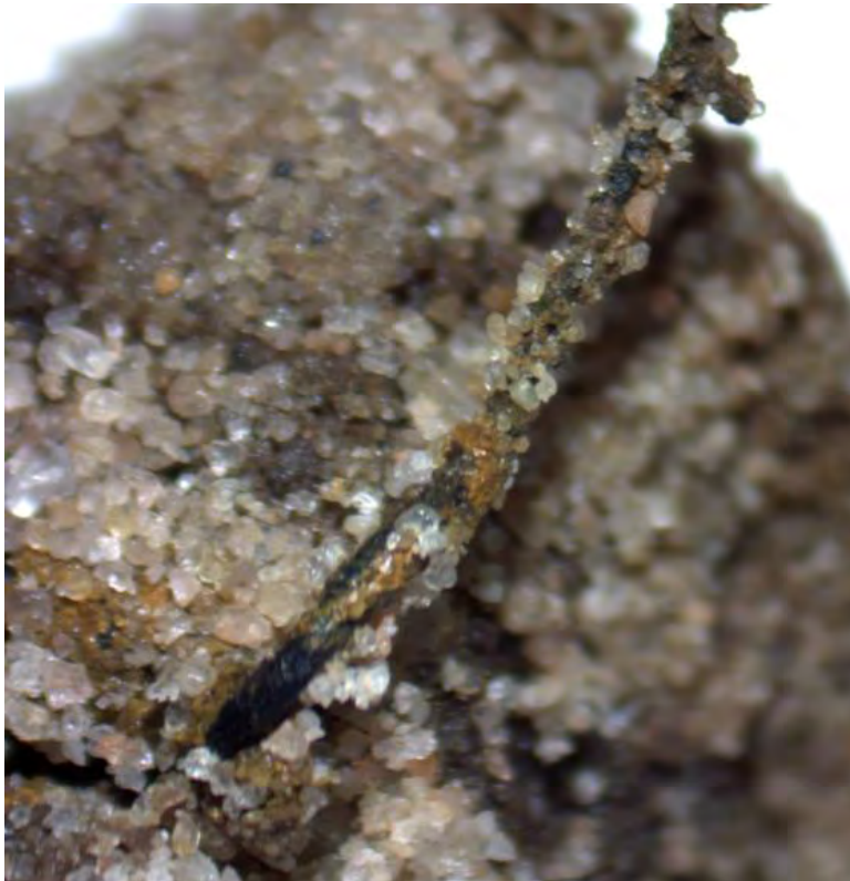
Figure 26. Fine (1mm) tree roots in sand/clay interface at 2.9m depth in LS31a.
