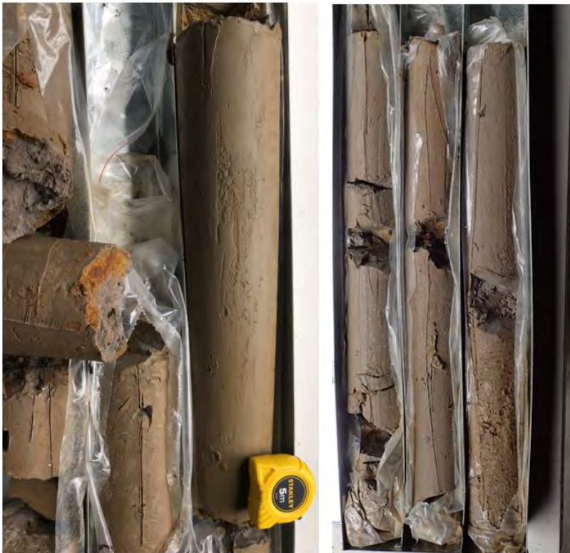
Figure 25. Massive sequences of high plasticity clays and sandy clays encountered during drilling Long Swamp 31 (Lake Broadwater). Note that incisions into the clay core are where samples have been collected for soil moisture and isotope sample analyses.
