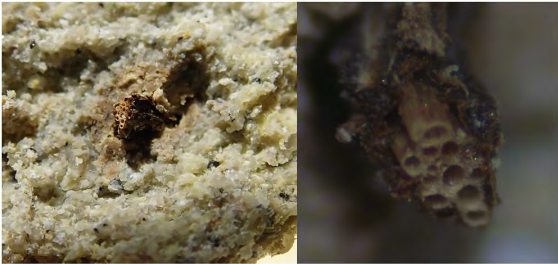
Figure 58. Open vessel structure of tree roots recorded at 7.6m in weathered Springbok Sandstone. Note water or resin droplets present within xylem in the photograph on the right.
