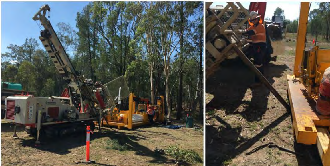
Figure 13. Angled core hole being drilled at the Glenburnie Study Site.
