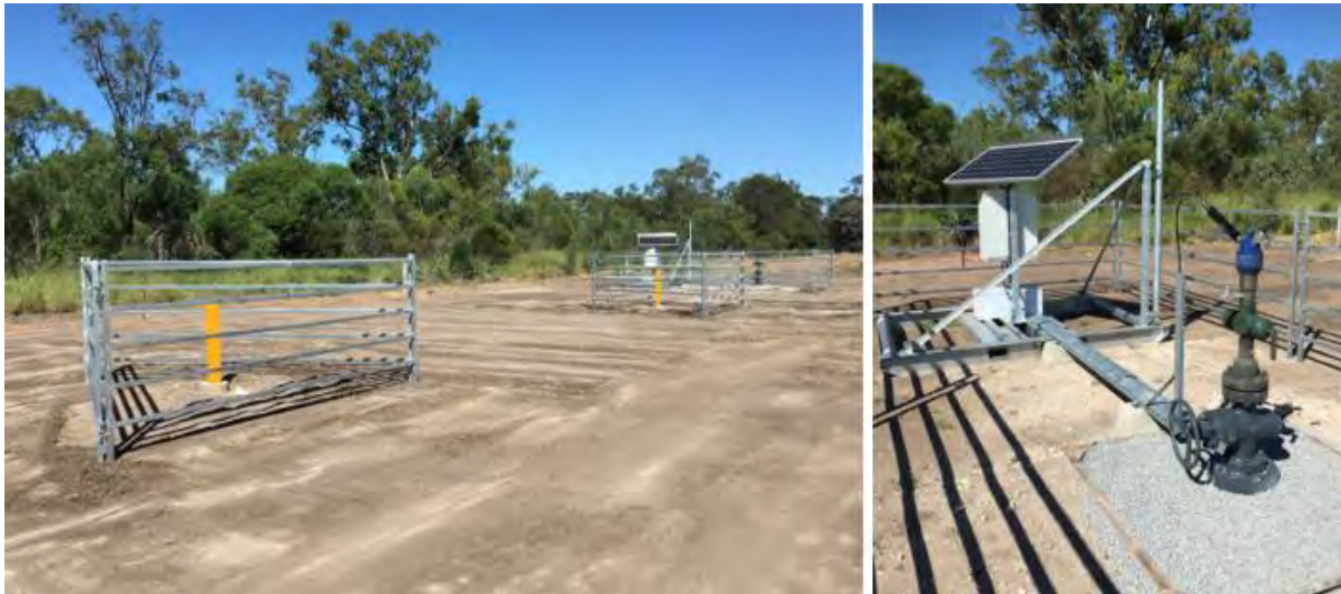
Figure 17. Nested deeper aquifer groundwater monitoring bores near Long Swamp 35 (Long Swamp 32, 33, and 34).
