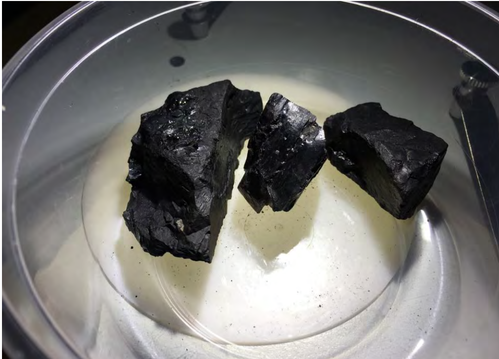
Figure 47. Coal seam and dull and bright coal samples (20mm thickness) collected from BL182A at 13.8m depth
