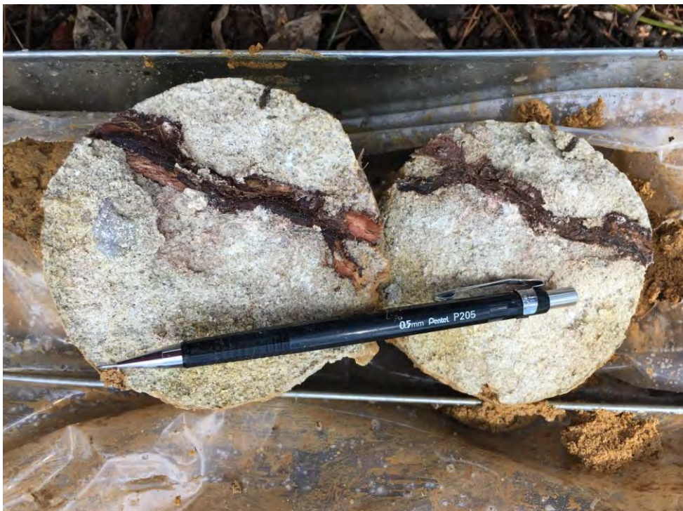
Figure 59. Large tree roots recorded penetrating along bedding in sandstone at 4.5mGL in GB20a.
