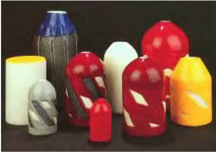
Plate 3-36: Pipeline cleaning pigs
