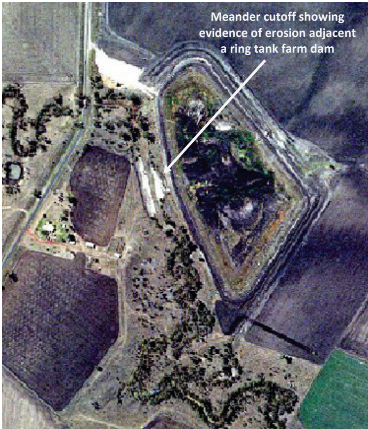
Figure A5-5. Example of a meander cutoff on the Condamine River (north branch)
