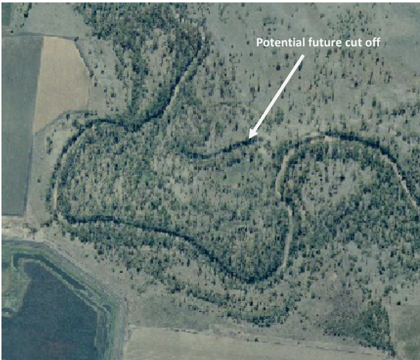
Figure A5-8. Example of potential cut off
